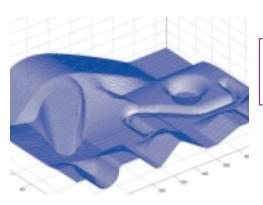
rating under Windows™, the "Path Optimizer", is also offered that takes an ISO part program generated by CAM as its input and generates as its output a group of fifth grade polynomials generated via appropriate numeric interpolation algorithms based on B-Splines. These polynomials that optimally describe the profile previously defined via points, are then executed directly by the CNC.
